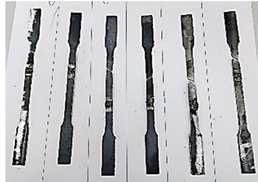
Fig. 11. Tensile specimen for welds performed with E6013 electrode after breaking.
