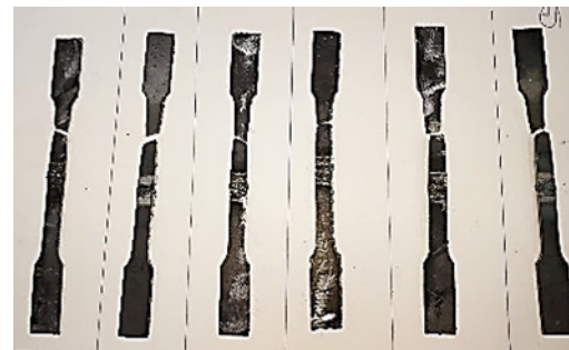
Fig. 12. Tensile specimen for welds performed with IMAN-8 electrode after breaking.
