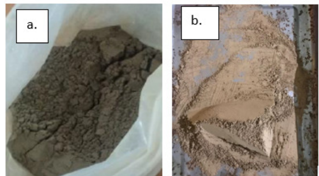
Fig. 1. a) Portland cement and b) FA from the Paiton power plant.
