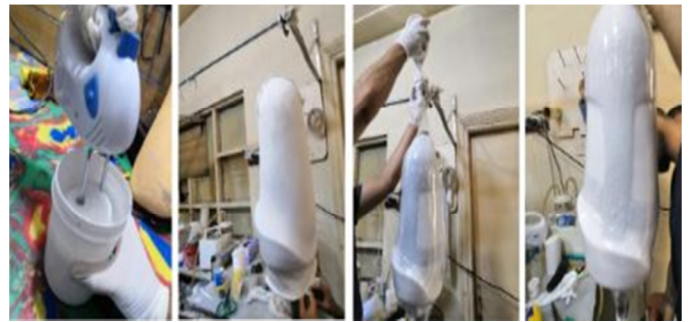
Fig. 5. Mixing of liquid silicon rubber with hardener and PVA addition.
