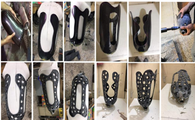
Fig. 4. Steps of cutting and smoothing the socket for manufacturing the required design of AK prosthesis.
