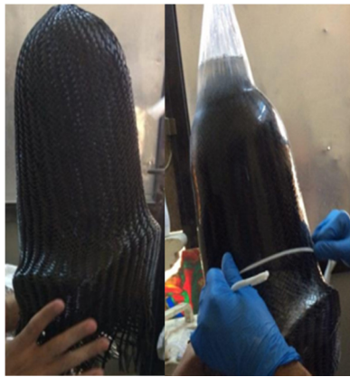
Fig. 3. Lamination used for manufacturing the AK prosthesis.
