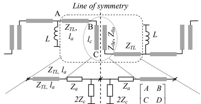
Fig. 3. Transmission line model of the Z-shaped EBG.
