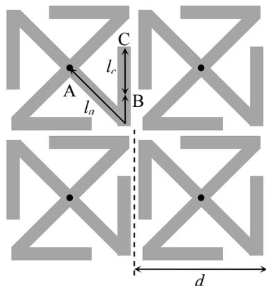
Fig. 1.  $2 \times 2$  periodic unit cells Z-shaped EBG structure.
