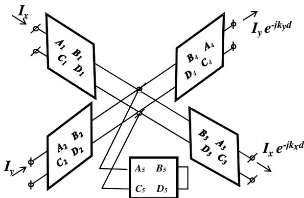
Fig. 2. Unit cell of a periodic structure, presented with the equivalent transmission matrices
