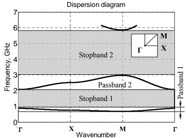
Fig. 4. Dispersion diagram for Z-shaped structure.
