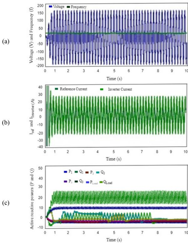
Fig. 7. GCM results: (a) Voltage and frequency, (b) reference and inverter currents, (c) active and reactive powers.
