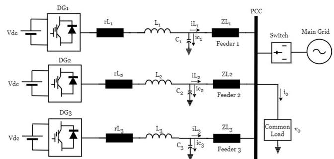
Fig. 1. A microgrid with three DG inverters connected in parallel.
