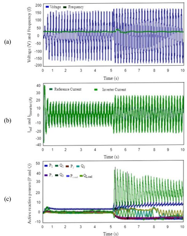
Fig. 10. Transition from IM to GCM: (a) Voltage and frequency, (b) reference and inverter currents, (c) active and reactive powers..
