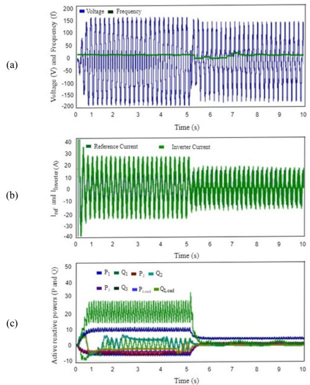
Fig. 8. Transition from GCM to IM: (a) Voltage and frequency, (b) reference and inverter currents, (c) active and reactive powers.
