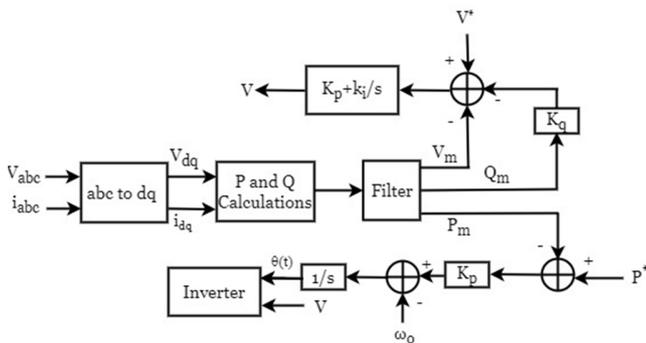
Fig. 4. Active and reactive power calculations.
