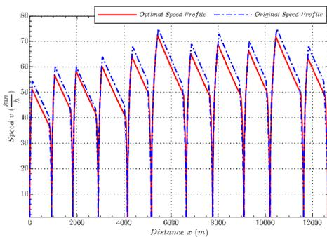
Fig. 1. Comparison of optimal and original speed profile without fixed-trip time.
