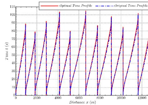
Fig. 2. Comparison of optimal original time profile without fixed-trip time.
