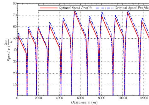
Fig. 3. Comparison of optimal and original speed profile with fixed-trip time.
