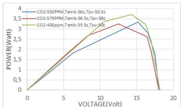
Fig. 11. Solar PV characteristics at 2 PM.
