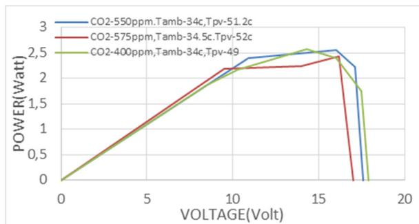
Fig. 13. Solar PV characteristics at 4 PM.
