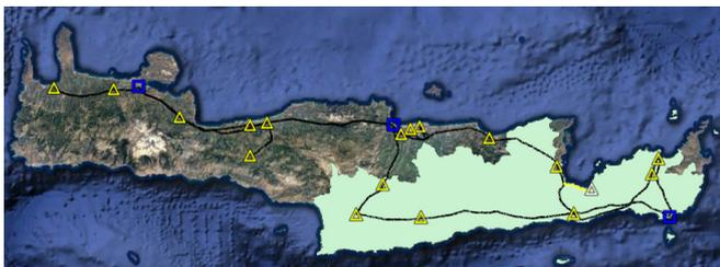
Fig. 6. Areas of Crete (with bright solid color) registered in the national Cadastre in 2019, including over 7,000 different easement cases and expropriated areas. Solid black lines depict the axes or overhead transmission lines, blue rectangles denote step up substations and yellow triangles denote step down substations. (Screenshot from Google Earth, DATA SIO, NOAA, U.S. Navy, NGA, GEBCO, Image Landsat / Copernicus).
