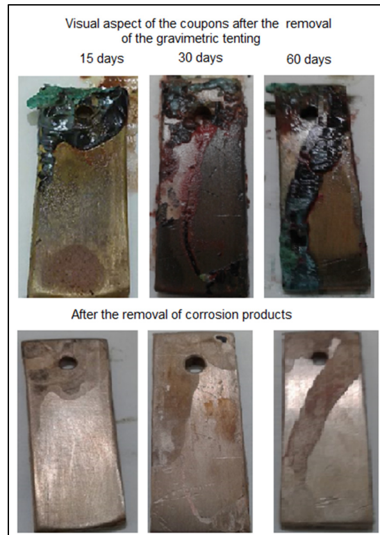
Fig. 6. Copper-nickel alloy coupons in gravimetric testing in saline solution with 5000mg/L sodium hypochlorite
