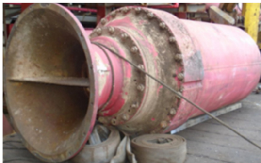
Fig. 2. Seawater suction pump
