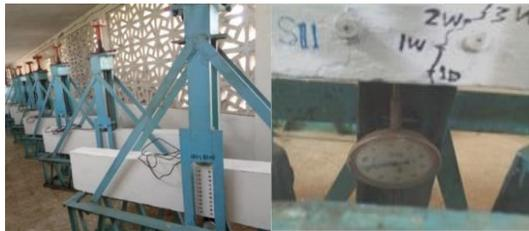
Fig. 3. Reinforced concrete beams for testing under long term loading.
