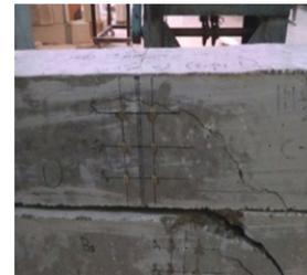
Fig. 6. Beam failure
